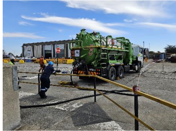
Photo 2: Good safety procedures on bunded areas during used oil collection.
